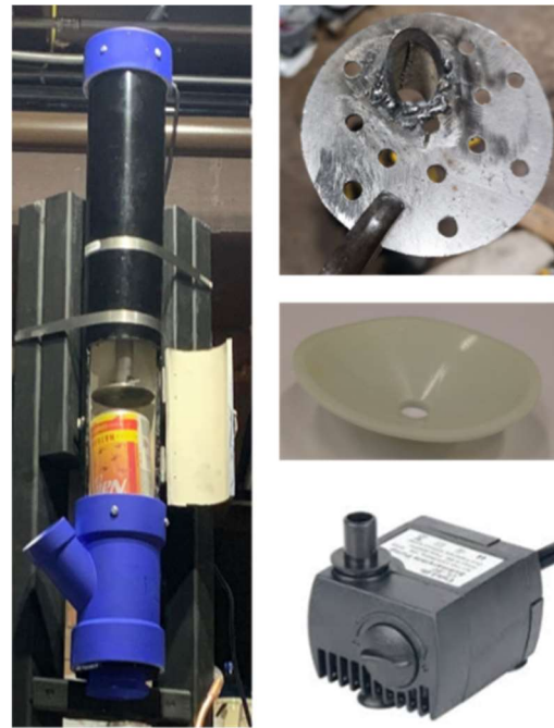
Fig. 7 PVC housing, puncture grate, 3D printed funnel, and the pump
