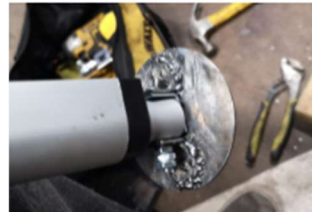
Fig. 5 Actuator with crushing plate attached to the end
