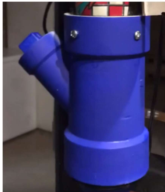
Fig. 6 Funnel reservoir w/ side funnel Note: the side funnel is capped off when not in use
