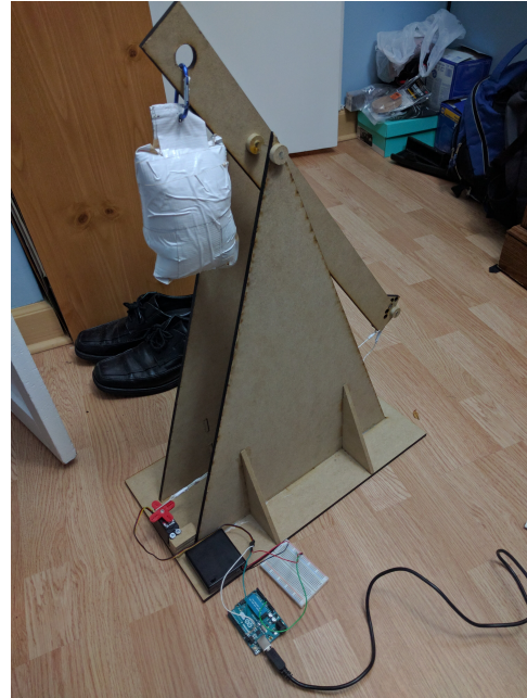
Fig. 1. Final assembled trebuchet with remote trigger release setup. The white bag was just a home made counter weight used to tune the trebuchet when the proper weight bags were not available.
